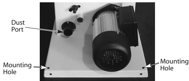
Figure 6- Mounting holes and dust port.
