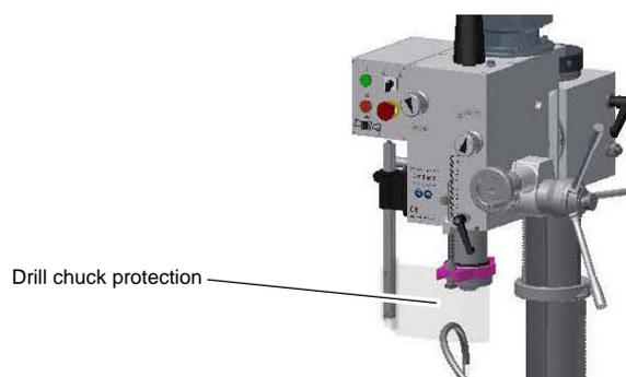
Fig.1-5: Drill chuck protection
