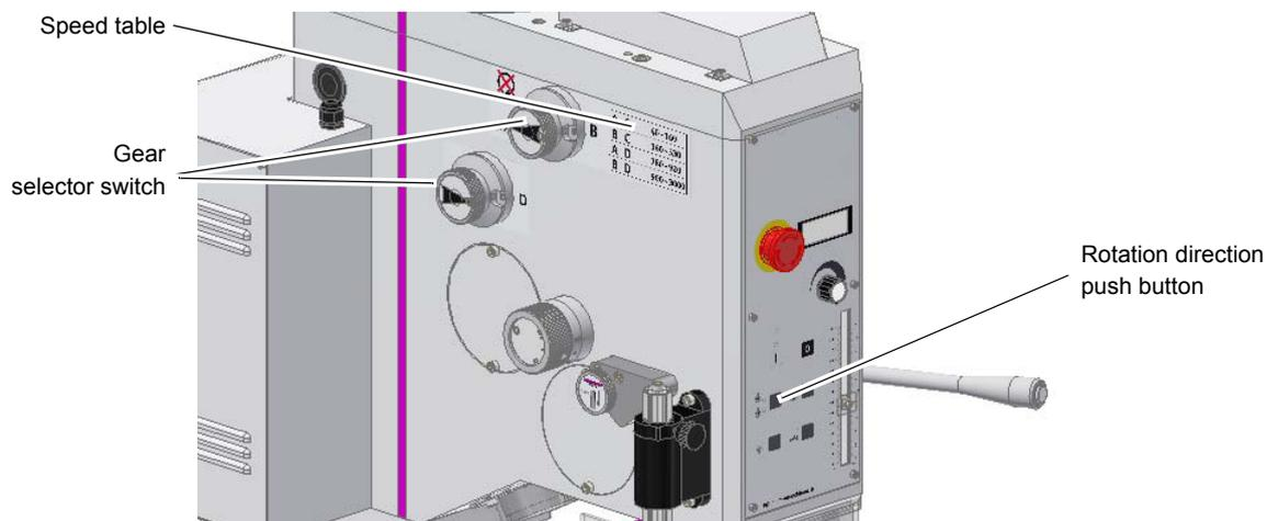
Img.4-13: Gear selector switch
