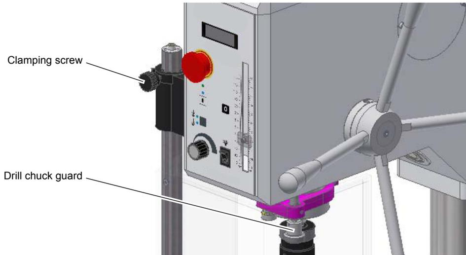
Img. 1-4: Drill chuck guard
