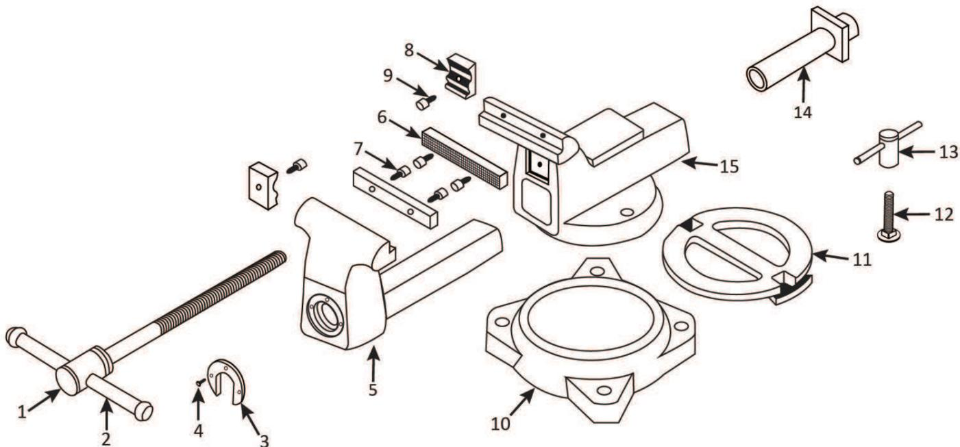
**Figure 1. Vice Exploded Parts View**
