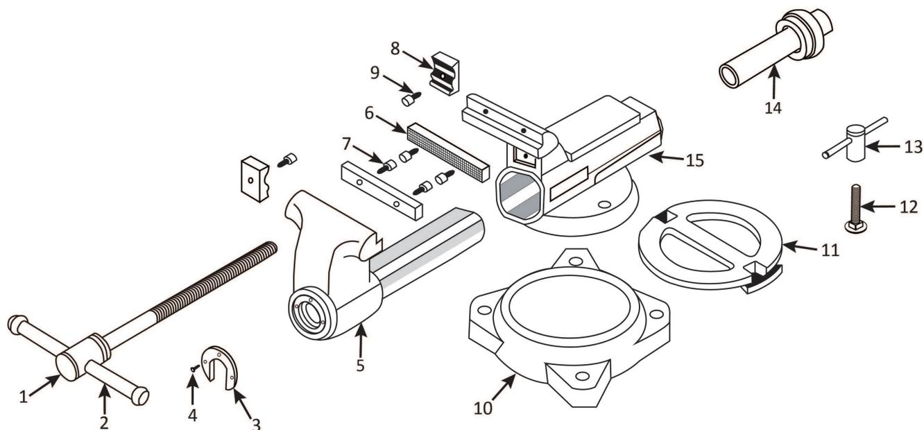
**Figure 1. Vice Exploded Parts View**
