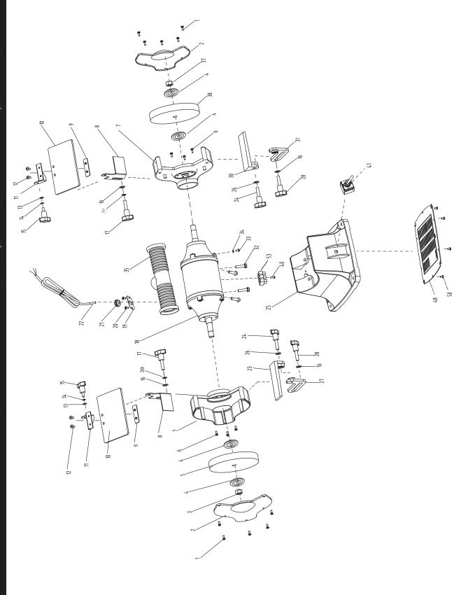
Figure 9 – Repair Parts Illustration for 9682102B, 10" Bench Grinder, 3 Phase
