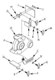
Figure 1 - Left Tool Rest and Eyeshield Assembly
