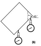
2) Select Plane XY. Key (ENT) |I|NE|-|X|Y| 3) Enter the angle of the angle surface  $\text{Key}(4) \rightarrow (5) \rightarrow (\text{BNT})$ ANGLE 45000 🖾 Key (₹ 4) Move the machine table along X axis. MOVEX Let the metering tool come just in contact with the working piece, and adjust the scale reading into zero, then move the machine table an arbitrary distance along X axis. 5) The moving distance on Y axis is displayed. Key (Y) 50690 🖾 MOVE
