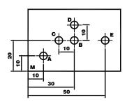
1) Let the Tool point to Point M reset under the absolute mode.
