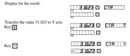
As shown in the figure, the distance AB=31.623, the tool is at Point A, move the machine table to bring the displayed value into zero, the position of Point B is reached, the processing of Hole B may start.
