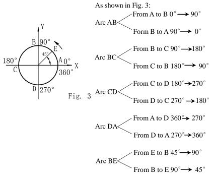
3) The procedure in using the Arc R Calculation function.
