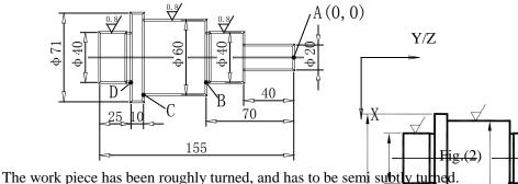
The unilateral allowance through rough turning is 0.05, the subtle turning
