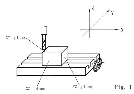
Let us recognize the plane coordinate and the start and end angles of a circular arc.
