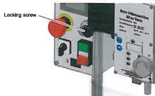
Fig. 1-3: Separating protective equipment
