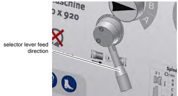
Illustr. 4-7: selector lever feed direction
