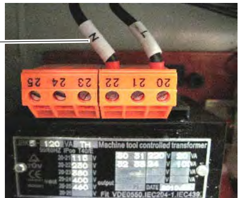
Illustr. 3-6: Transformer wiring
